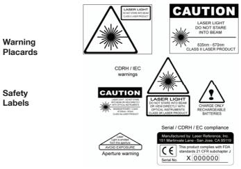
**Note:** The AlphaR is a CDRH class II laser and an IEC 60825 class 2 laser. It conforms to applicable EC directives regarding RFI and EMI, and to FDA performance standards 21 CFR subchapter J.
